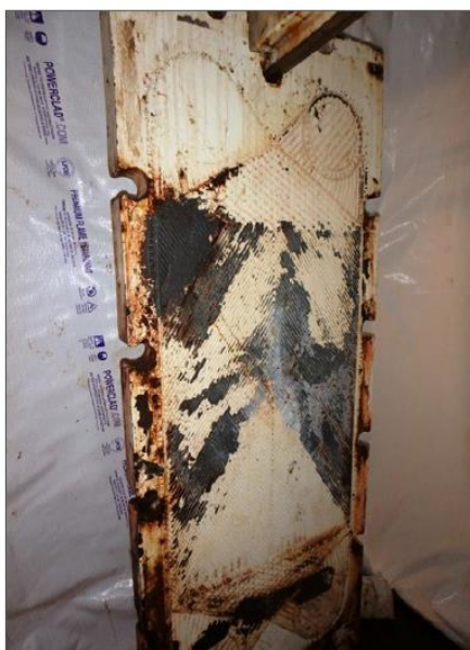
Backplate of cooler prior to repair
