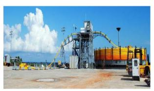
We designed a fully scalable carousel system that can be manufactured to handle 1,000 MT or up to 9,000 MT for the largest carousel, depending on customer requirements. The carousels can be used for land-based storage or offshore deployment of product from an installation vessel.
