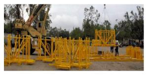
Deep Down's Rapid Deployment Cartridges (RDC) and Subsea Deployment Baskets (SDB) provide installation contractors with safer methods to install umbilicals and flying leads. Both the RDC and SDB provide storage, transportation, and installation methods for your flexible pipe and umbilical flying leads. The RDC and SDB are stackable and typically
